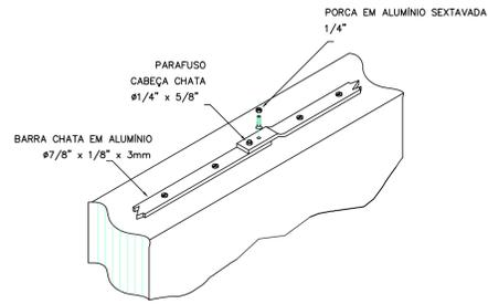
DETALHE DE EMENDA DA BARRA CHATA NA ALVENARIA
